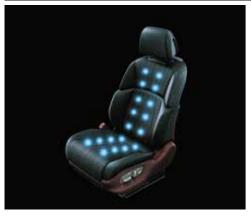
Air bladders integrated into the seatback and seat cushion are inflated to apply pressure from the occupant's back to the thighs, contributing to a feeling of relaxation. Programs can be selected for the entire body as well as particular areas (Upper Body, Lower Body and Lumbar).
