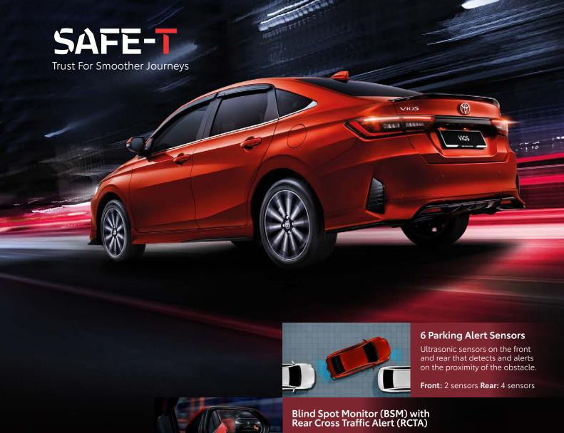
Detects and alerts of vehicles within the driver's blindspot. Alerts driver of oncoming vehicles from the rear when the reverse gear is activated.
